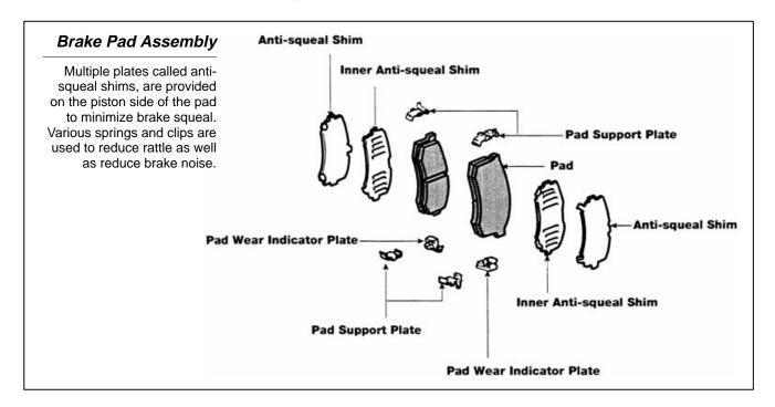
The brake pad material is bonded to a stamped steel backing plate with a high temperature adhesive to which heat and pressure are applied to cure the assembly. A slit is provided on the face of the pad to indicate the allowable limit of pad wear and provide a path for brake dust and gas to escape.
